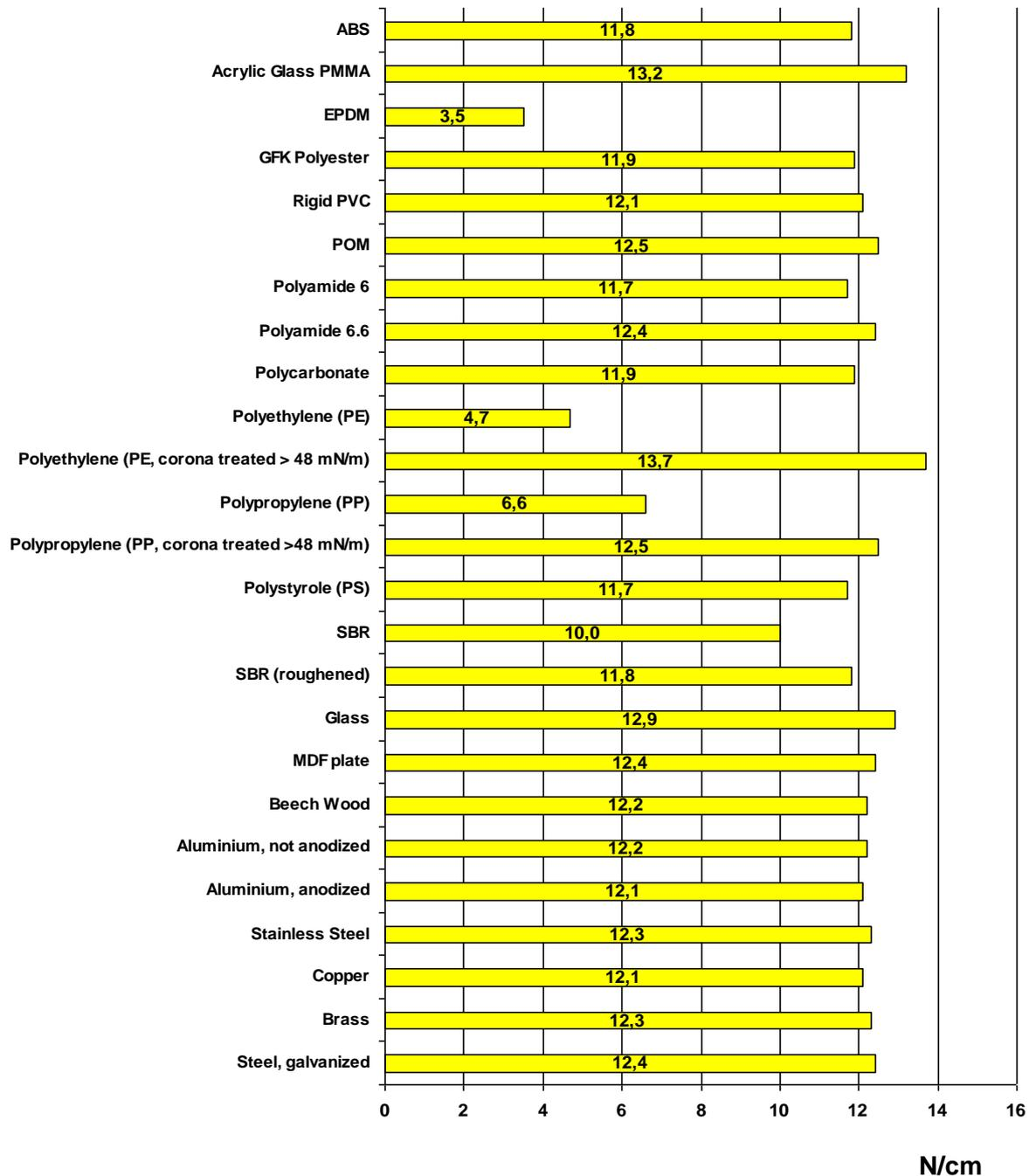
Tested according to PSTC 1. Measured with peel tester type L 500 from Lloyd Instruments. Load cell 100 N, class 1, DIN EN ISO 7500-1 for tension and pressure, peel angle: 180°, printed with 21-140(T) on 125 µm polycarbonate film, measured after 72 h-storage at normal climate (according to DIN 50014-23/50-1). Peel speed 300 mm/min. Applied with a hand roller (according to PSTC standard: 10 pounds, rolled 5x in each direction). Adhesion area: 2,5 x 10 cm. N/inch.
