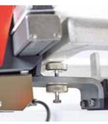
Frame profile height adjusting screw of SEFAR® 3A
