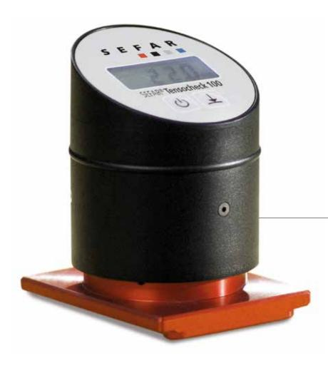
SEFAR® Tensocheck 100 is an electronic gauge for monitoring screen tension. Its outstanding advantages: Its excellent value for money and ease of use without requiring previous experience. SEFAR® Tensocheck 100 is also available having a serial port for connection to SEFAR® 51i. Your advantage: Fully automatic, precise tensioning at preselected values in N/cm (Existing devices not having an interface are not able to be converted).
